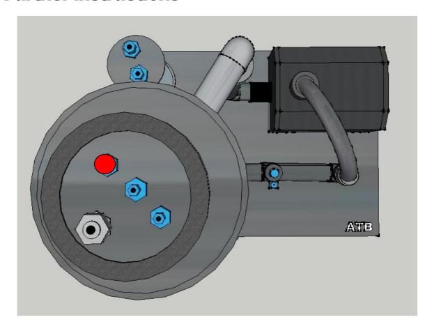
After the ca-reactor is filled with media and you fill in the water, you should remove the red hose from the top of the ca-reactor. Then the air can come out. You can connect the hose again after the water is coming out.
